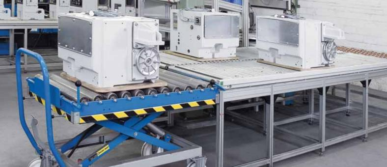
Moving heavy production parts safely along the assembly line with minimal effort.
