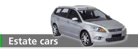
In estate cars and hatchbacks, existing manufacturer's fixing points are used to secure the mounting platforms into position. Easy access to materials and spare parts is gained via the rear and side doors of the vehicle.
